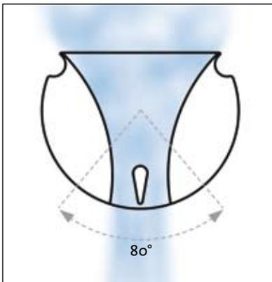
The secret of EVOLVENT®. The air flow is compressed, concentrated and accelerated in the nozzle. A turbulence-free, uniform air curtain is created with a high shielding capacity.
