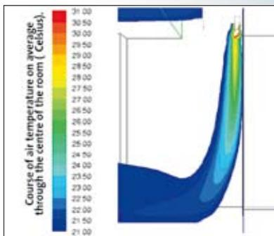
The operating principle of air curtain systems underwent scientific studies in a test chamber within the scope of a university thesis completed at the Institute for Technical Building Infrastructure of the Faculty of Process Engineering, Energy and Mechanical Systems at Cologne University of Applied Sciences.
